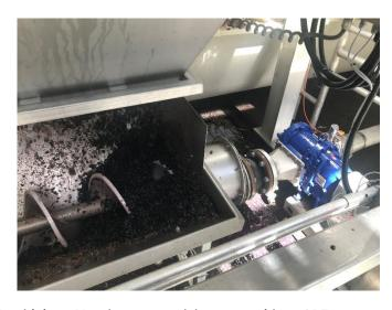
Combining a Vogelsang rotary lobe pump with an OPE screw sump provides an unmatch package for your Must pumping requirements. Packages can provide up to 60 tons per hour in both mobile and stationary designs.
